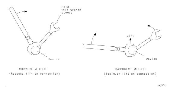
**4.** Hold the torque wrench lightly, at the end of the handle only (beyond the groove). See Figure 3-8
