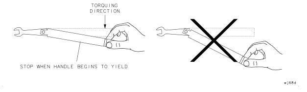
**5.** Apply downward force perpendicular to the wrench handle. See Figure 3-8. This applies torque to the connection through the wrench.
