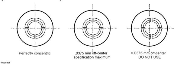
Figure 3-4 Concentricity of a Male Connector
